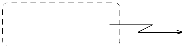
Figure 258 - InterruptibleActivityRegion notation with interrupting edge
